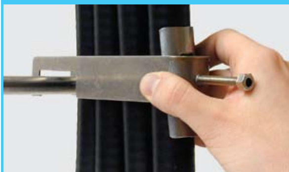
3 Insert the interlayers between the cables and the holder
